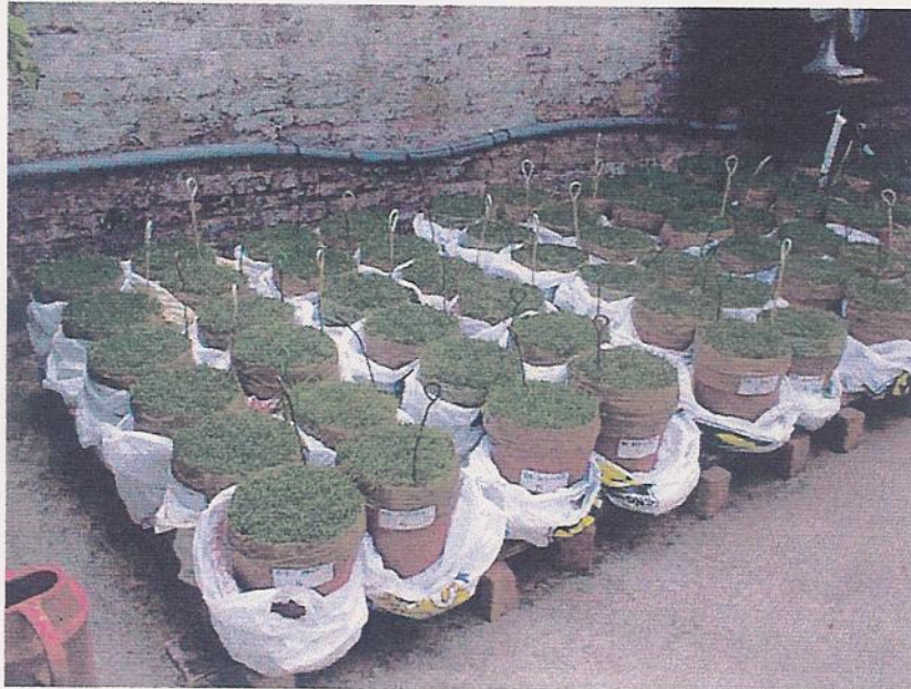
PLATE 4 Four sand rootzone lysimeters illustrating the contrast between swards with and without Fytogreen amendments and between irrigation regimes (30 June 2000). Top row = 10mm irrigation, bottom row = 0mm irrigation. Left column = no Fytogreen, right column = Fytogreen
